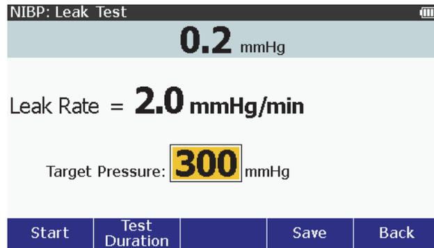
Figure 38. Example Leak Test Result Screen
