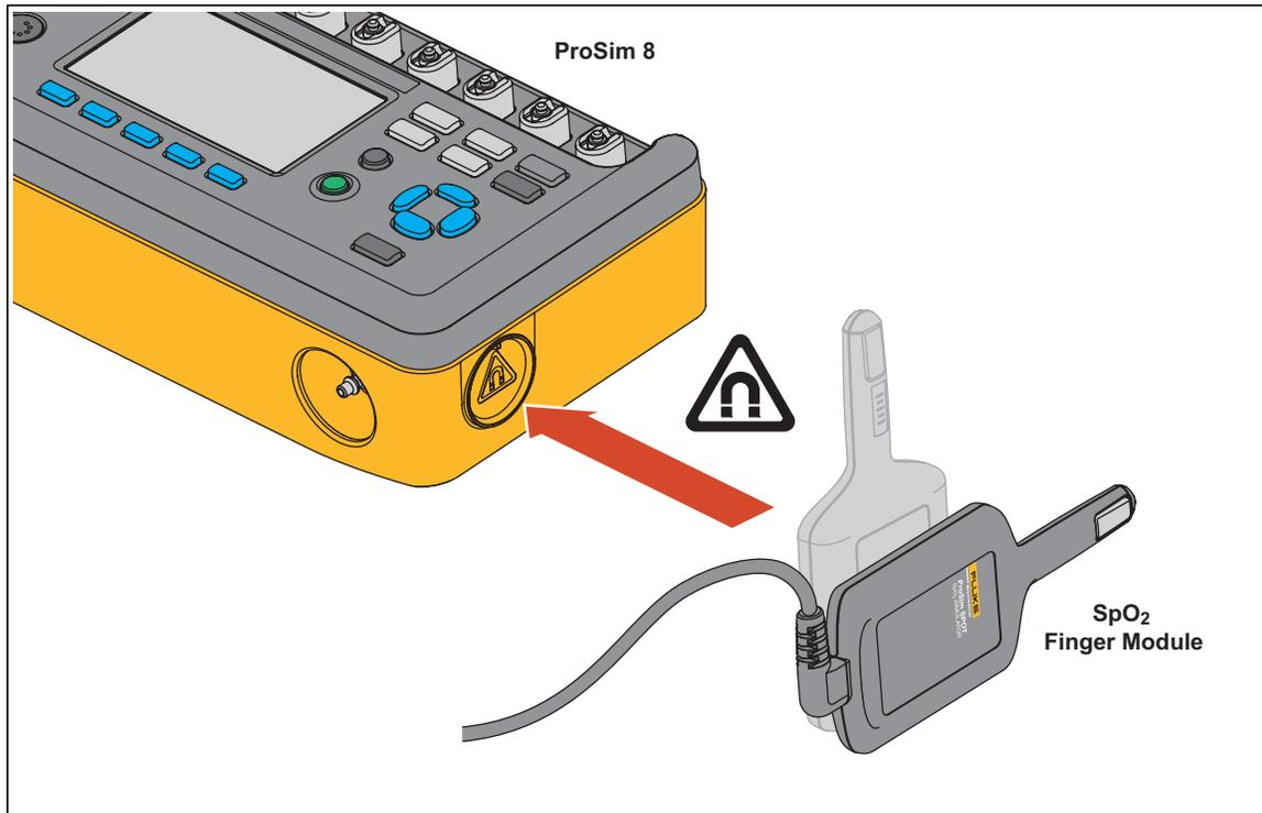
Figure 47. Magnetic Holder for SpO<sub>2</sub> Artificial Finger
