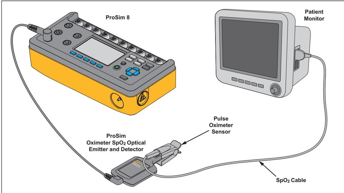
Figure 45. Oximeter SpO<sub>2</sub> Optical Emitter and Detector Connections
