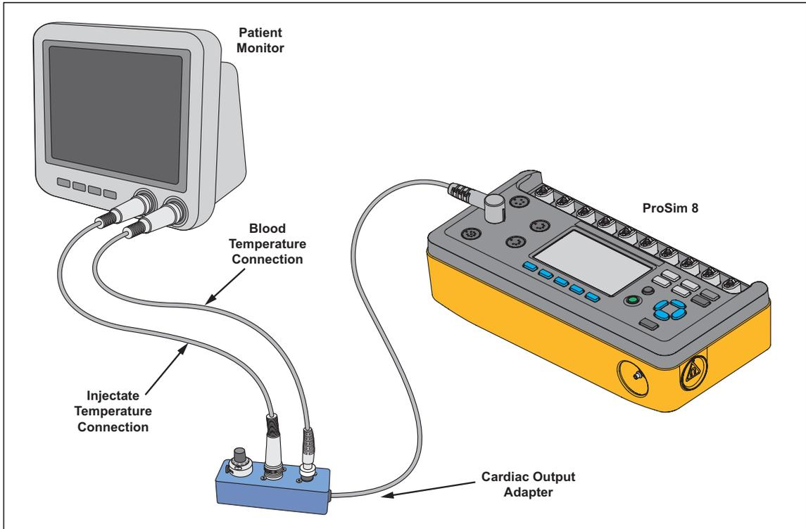
Figure 27. Cardiac Output Connections
