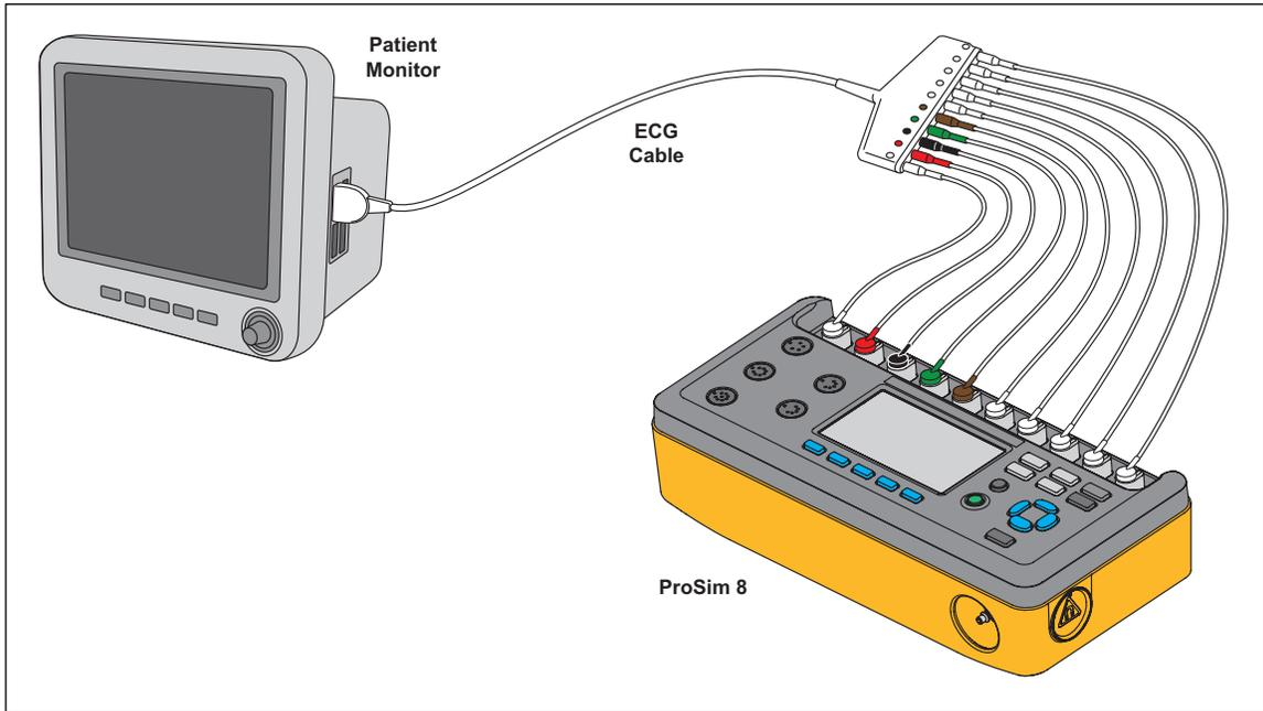
Figure 4. ECG Connections
