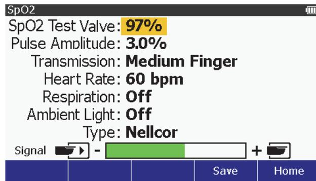
Figure 44. Oximeter SpO<sub>2</sub> Optical Emitter and Detector Screen
