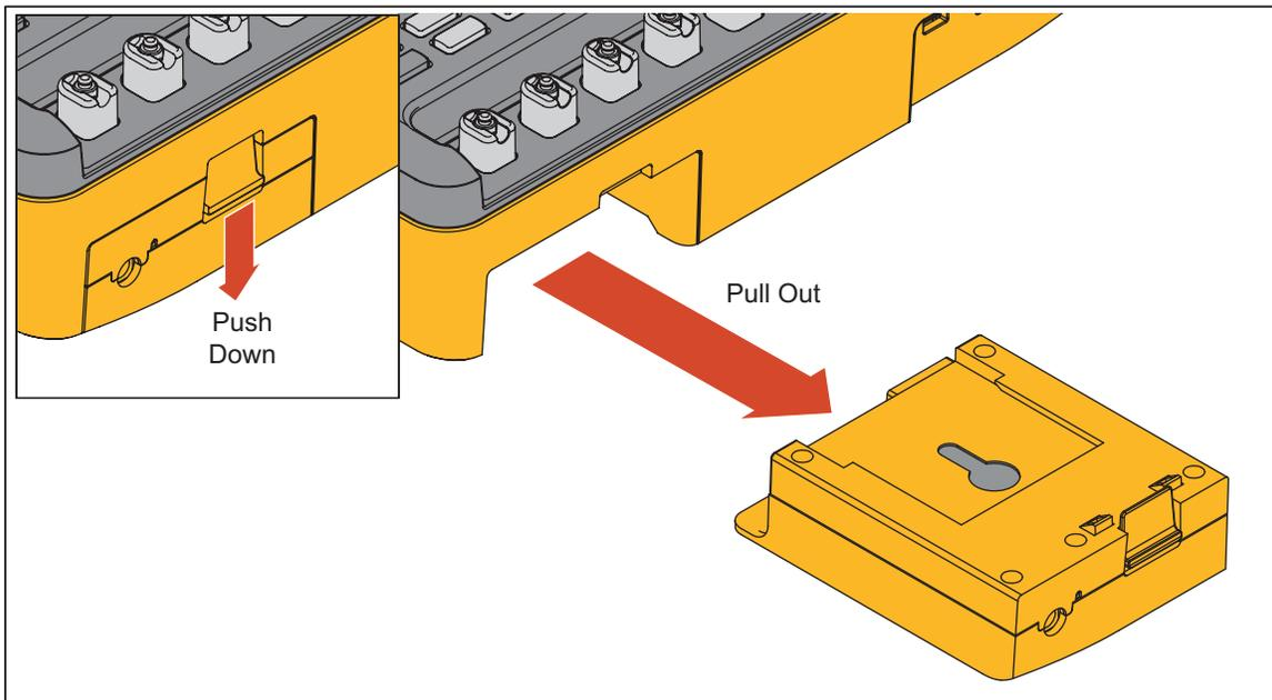
Figure 61. Battery Removal
