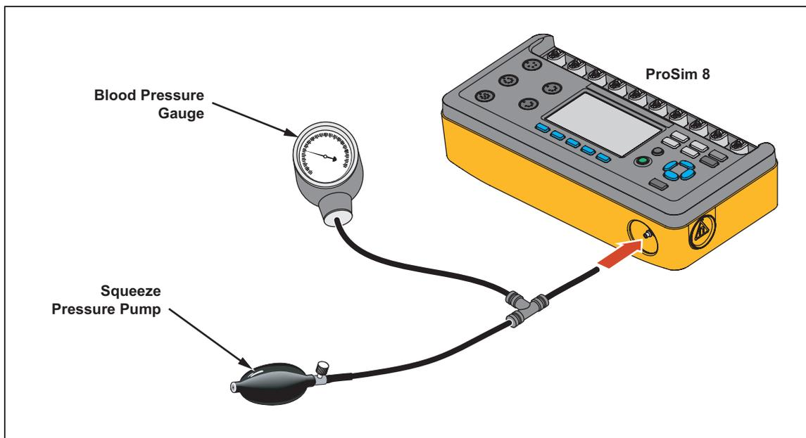
Figure 42. Manometer Connections
