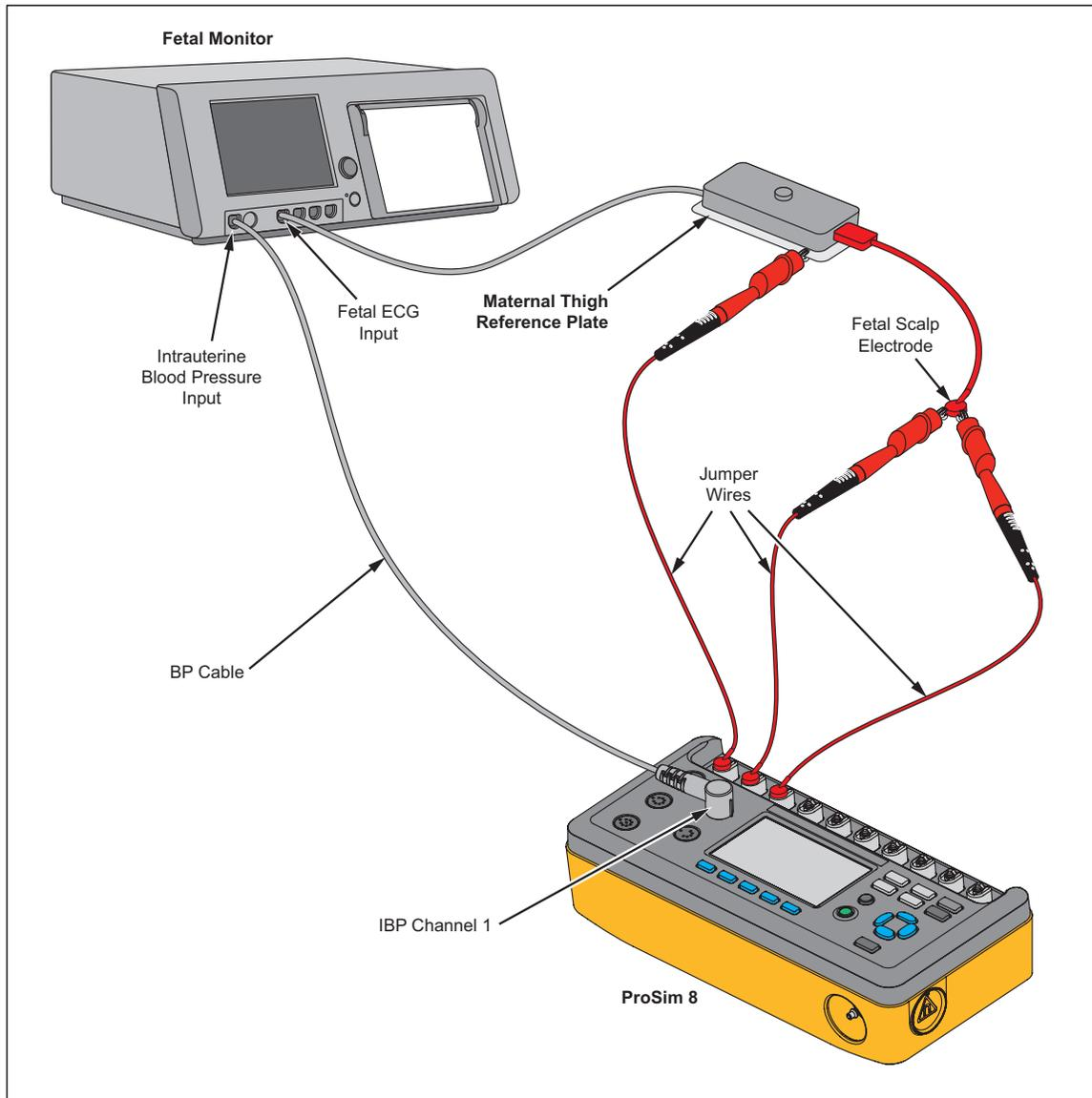
Figure 13. Fetal Monitor Connections for Intrauterine Pressure Simulation
