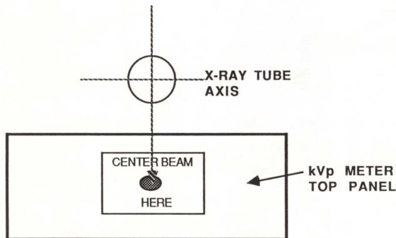
*Figure 3-1. Detector Positioning*
